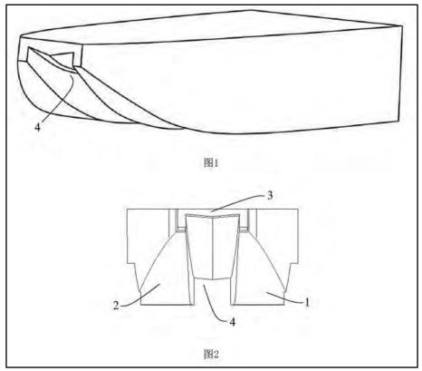
Figure 15: Diagrams of the proposed amphibious vehicle hull design depicting the left, right, and central vehicle bodies (Source: Google Patents)<sup>119</sup>
