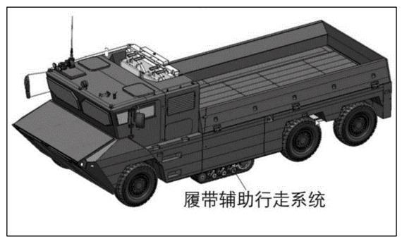
Figure 19: Diagram depicting the proposed auxiliary crawler system on a very likely amphibious logistics vehicle (Source: Google Patents)<sup>154</sup>
