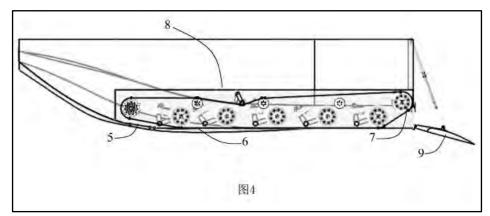
Figure 16: Diagram of the proposed amphibious vehicle hull design depicting the retractable tracks, sealing plates, and stern flap (Source: Google Patents)<sup>120</sup>
