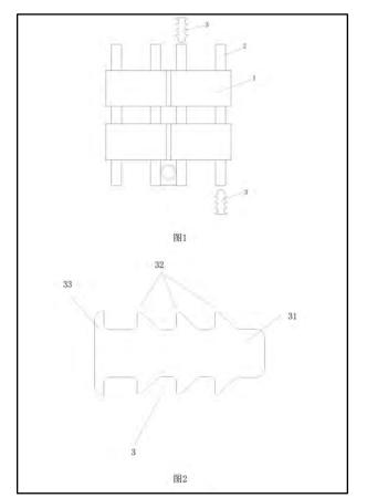
Figure 18: Diagram of the proposed track pin plug design (Source: Google Patents)<sup>146</sup>
