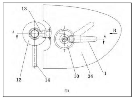
Figure 20: Diagram of the proposed rear gate locking and sealing mechanism (Source: Google Patents)<sup>163</sup>
