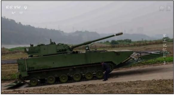
Figure 4: The Type-05 with its bow and stern flaps unfolded (Source: CCTV<sup>59</sup>)
