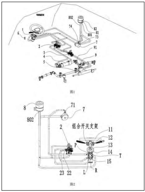
Figure 21: Diagrams of the proposed integrated steering system (Source: Google Patents)<sup>175</sup>
