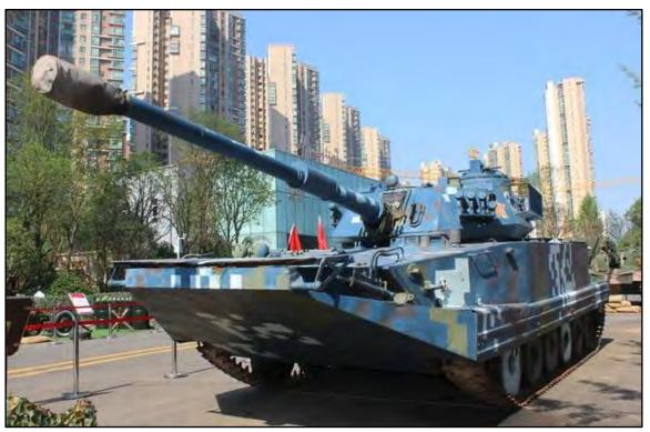
Figure 10: The Type-63A amphibious assault vehicle (Source: Hunan Today<sup>73</sup>)
