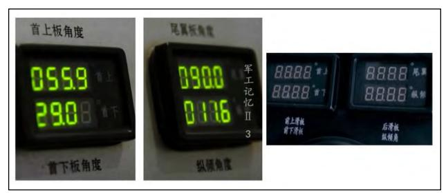
*Figure 6*: Experimental Type-05 gauge showing upper and lower bow flap angles (left); experimental Type-05 gauge showing stern flap angle (center); Type-05 gauge likely showing upper and lower front bow angles and stern flap angle (right) (Source: CCTV<sup>61</sup>)
