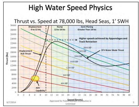
*Figure 5*: Graph of HWS physics that depicts the engine horsepower requirements to move from the speed hump to the semi-planing state (Source: Concept Exploration of the Amphibious Combat Vehicle<sup>60</sup>)
