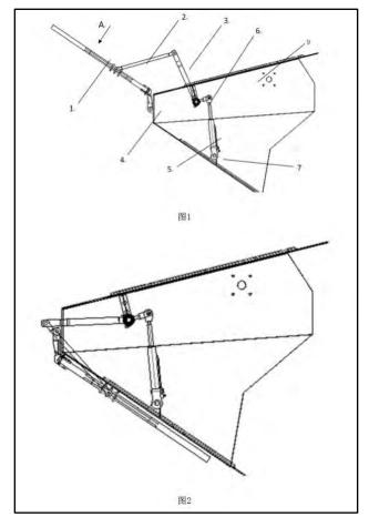
Figure 17: Diagrams of the proposed bow flap design (Source: Google Patents)<sup>131</sup>
