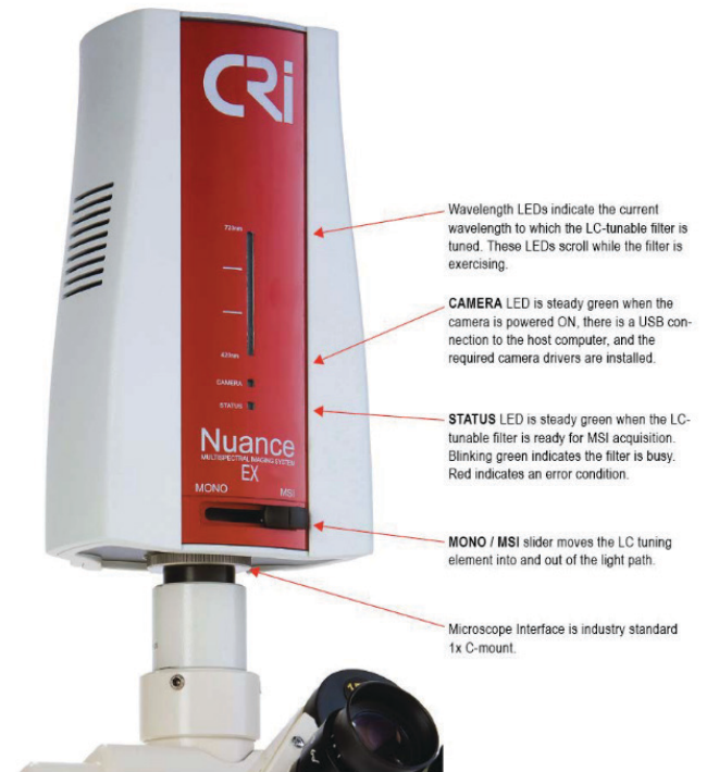
Figure 4: Nuance EX multispectral imaging system from PerkinElmer (Source: PerkinElmer 122 )
